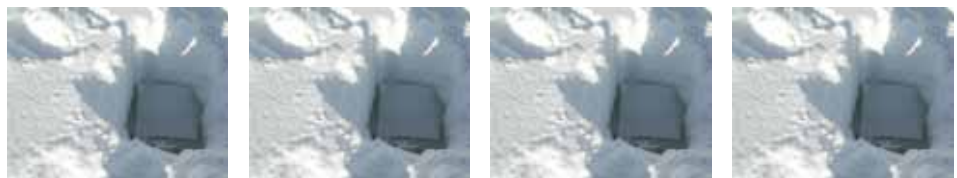
Remote control avalanche beacon transmitters with a probing surface of 40 by 60 centimeters
