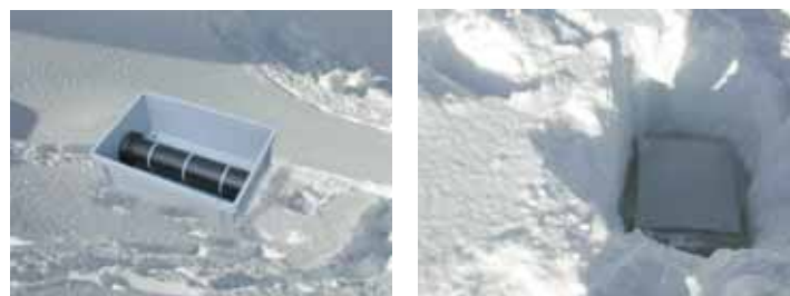
Avalanche Transmitter RTX 457 LT with target for probing
