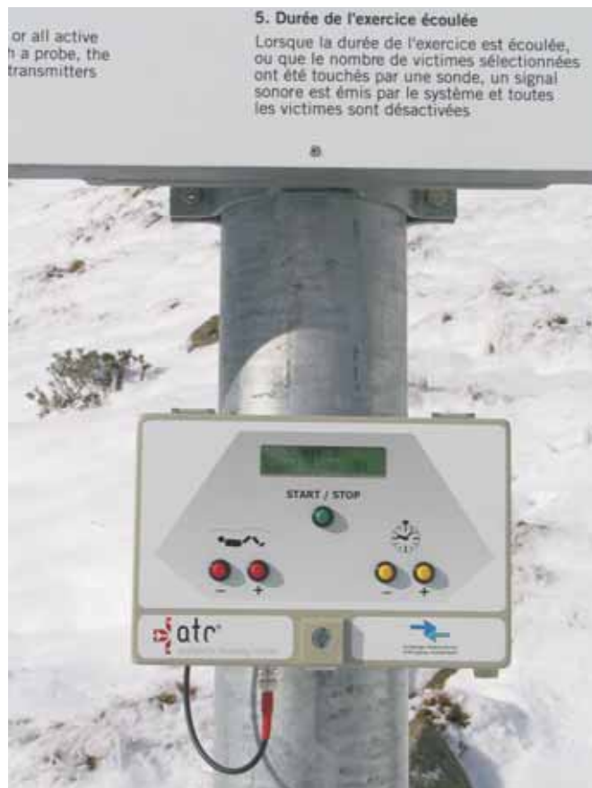
Permanently installed control unit FCU for 16 avalanche transmitters with indicators for the currently activated transmitters including probing hits
